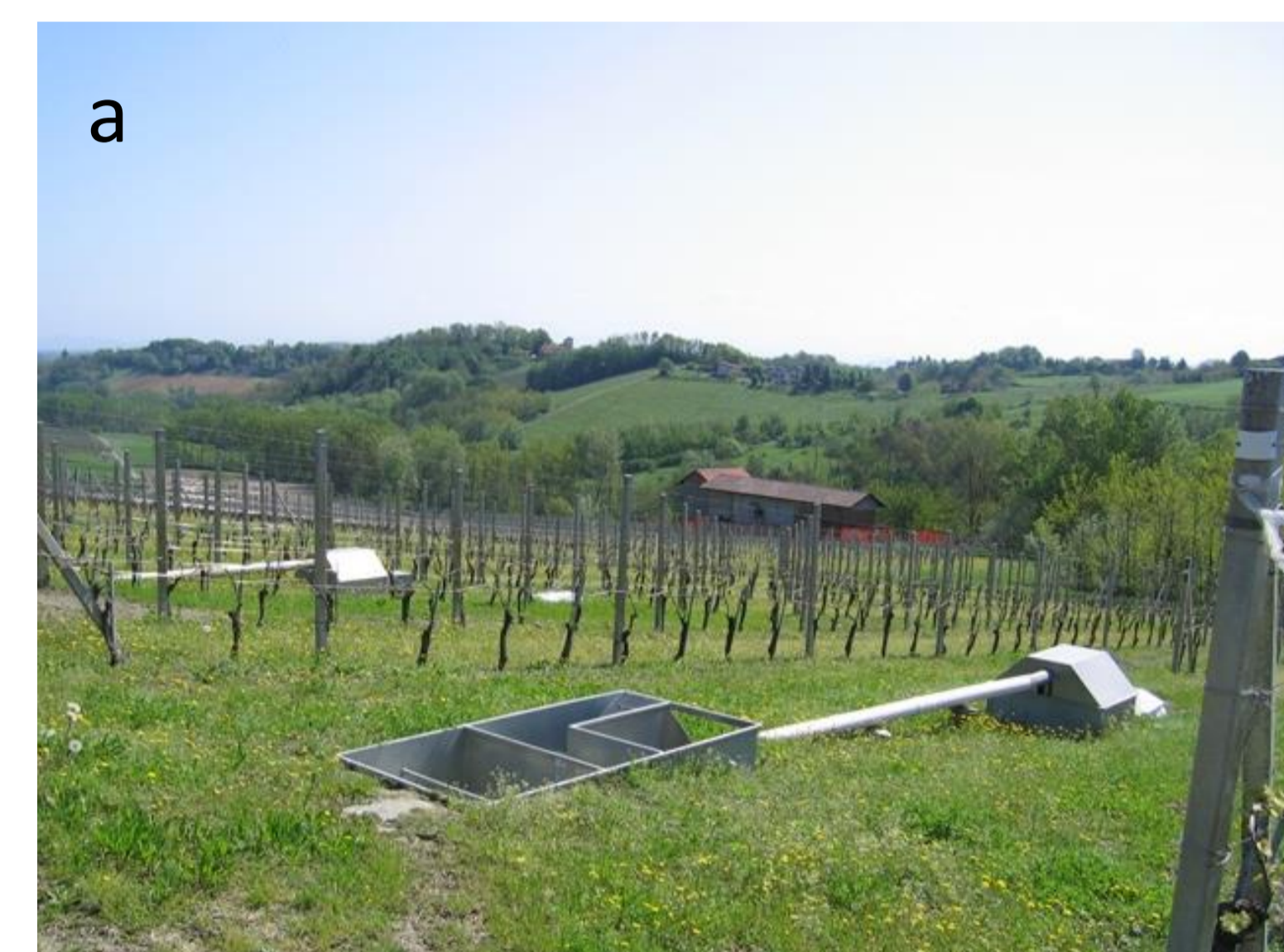
Fig. 2. The runoff measuring system: a) sedimentation traps and tipping bucket at the Tenuta Cannona Experimental Site; b) details of the tipping bucket system
